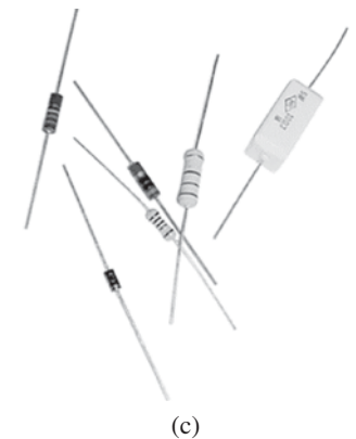
FIGURE 2-2 The resistor: (a) Circuit symbol. (b) i-v characteristics. (c) Carbon or film resistors. (d) Wire-wound resistors.
